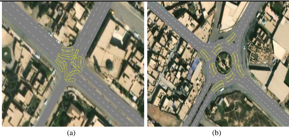
Fig 3. (a) Reduce Speed Areas in the Unsignalized Intersection. (b) Reduce Speed Areas in the roundabouts.
