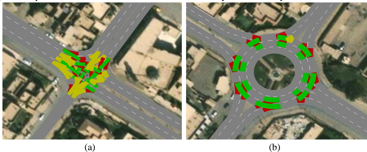
Fig 4. (a) Conflict Areas in the Unsignalized Intersection. (b) Conflict Areas in the roundabouts.
