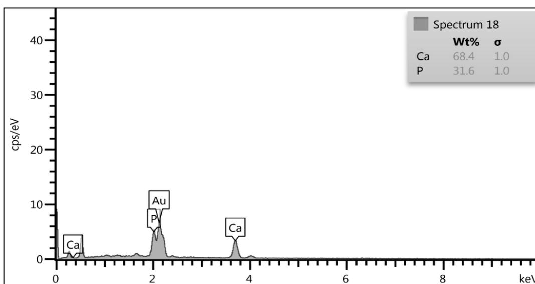
Figure 3: EDS spectrum for calcined bone powder at 800 °C calcination temperature
