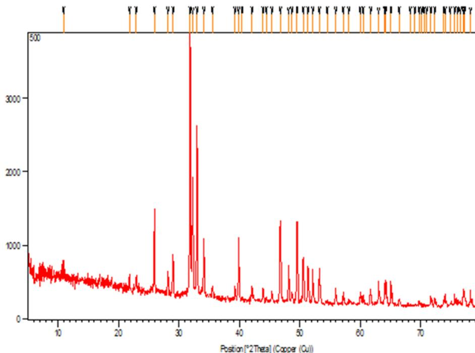
Figure 4-B: XRD spectra of calcined bone powder at 800°C
