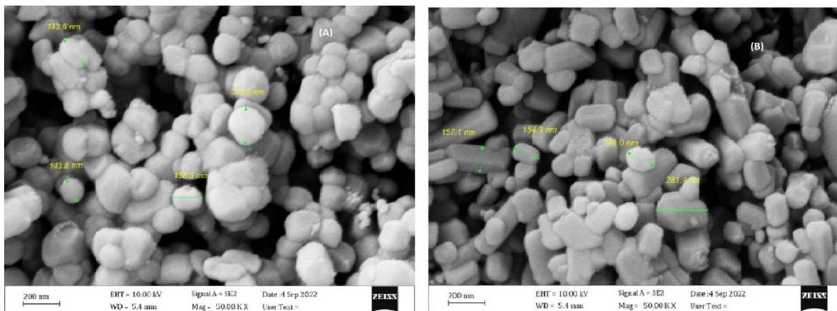
**Fig. 4: A and B: FE-SEM images of HAp with scale equal to 200 nm**
