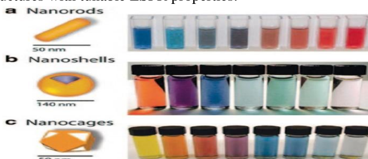
Figure 1.8. Metallic nanostructures with tunable localized surface plasmon resonance (LSPR): a - Au nanorods with different aspect ratios, b – Au nanoshells with different shell thicknesses, 1 and c – Au/Ag nanocages with different compositions and shell thicknesses (reproduced with
