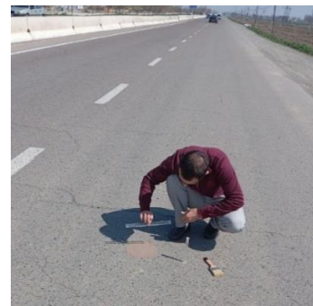
Figure 3. Pavement texture measurement process and view of a formed patch
