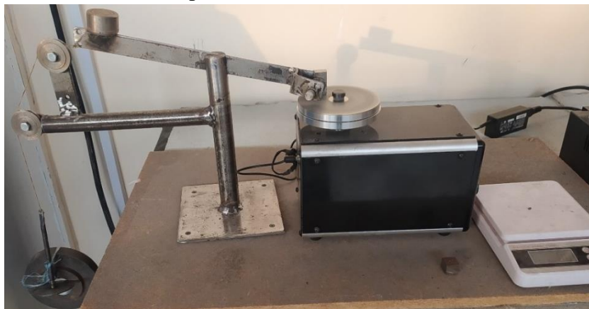
Picture 2. General view of a special device with a diamond disc for determining the wear resistance of samples
