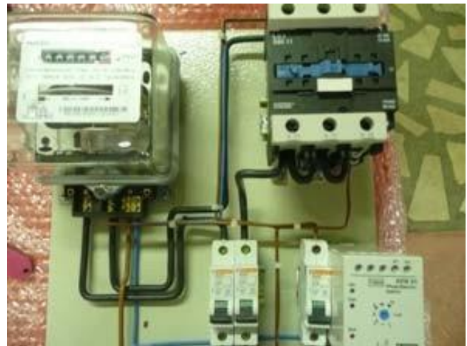
Figure 2. Control of street lights through photocells
