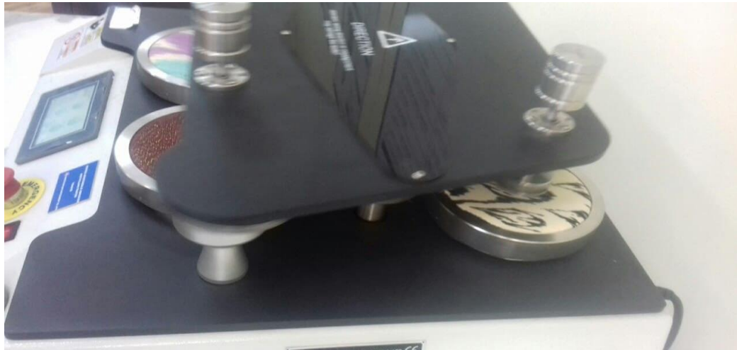
Figure 6. The process of testing samples for abrasion resistance.
