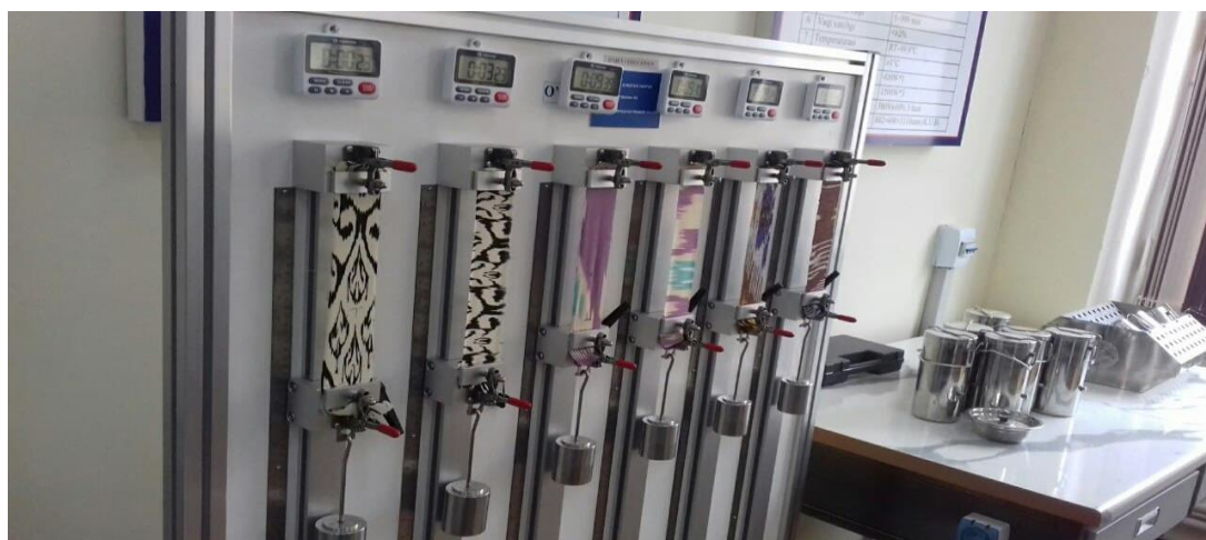
Figure 9. Fabric Elongation at Break Testing Process
