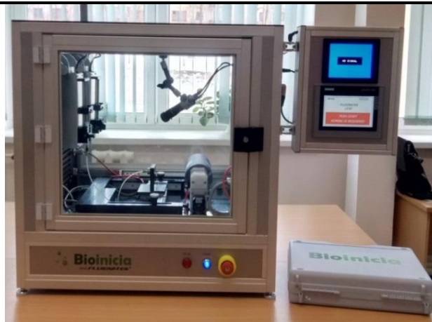
Fig. 1. External view of the laboratory electrospinning system.
