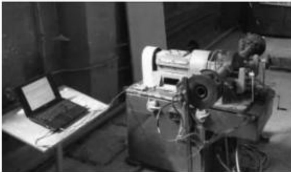
Figure 1. Test stand for the vibroacoustic diagnostics of passenger car driving axles
