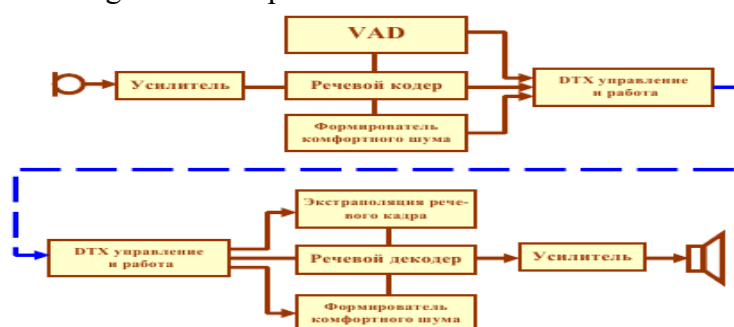
Рис. 1. Structural diagram of speech processing processes in the standard GSM.
