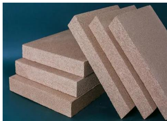
Picture 3. Golden colored expanded vermiculite and vermiculite boards based on the basis of expanded vermiculite
